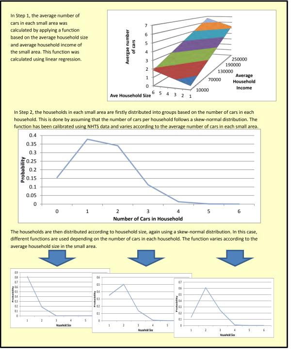
Figure 8 Disaggregate Model Description
