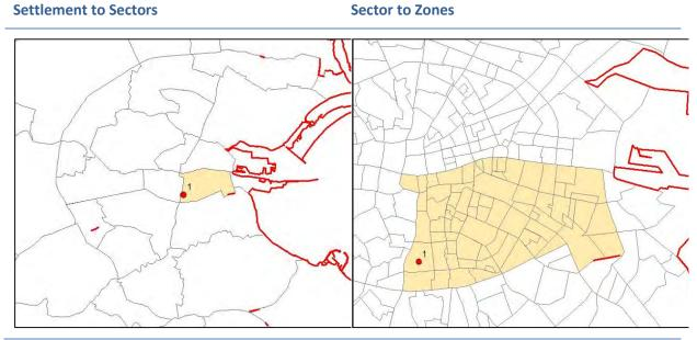
Figure 15 Example of Two Step Approach to Disaggregating Sectors to Internal Zone
